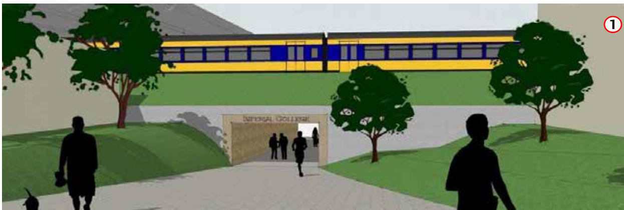
Figure 3.28: Northern crossing (1): Shallow pedestrian underpass
